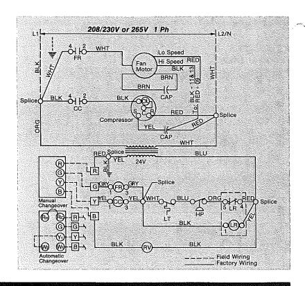
Wiring Diagram for Horizontal MODELS 19 - 61 208/230V or 265V Single Phase Power
