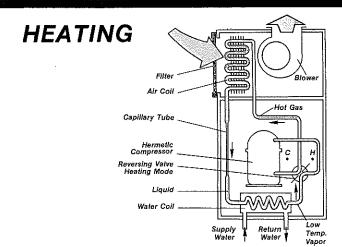
On demand for HEATING, the thermostat activates the blower and positions the reversing valve into the heating mode.
