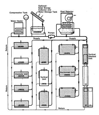
The CHP system consists of multiples of water source heat pumps connected in parallel by a two pipe closed loop through which water is circulated to each unit. The temperature of the water is maintained between 60°F and 90°F by means of a water heater which prevents the temperature from dropping below 60°F and a heat rejector which prevents the temperature from exceeding 90°F.
