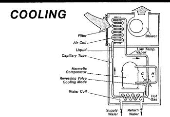
Upon demand for COOLING, the thermostat activates the blower and positions the reversing valve into the cooling mode.
